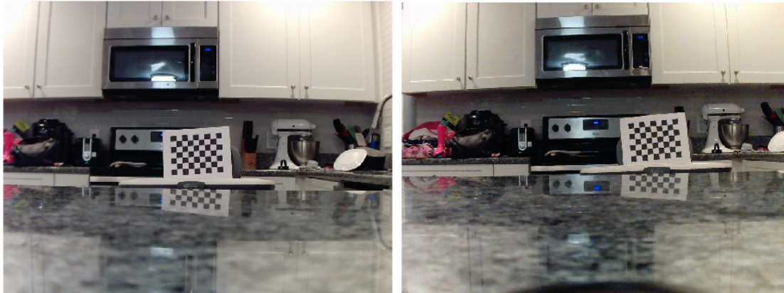
Figure 9A.1: Stereo images used to complete camera system calibration in MATLAB
